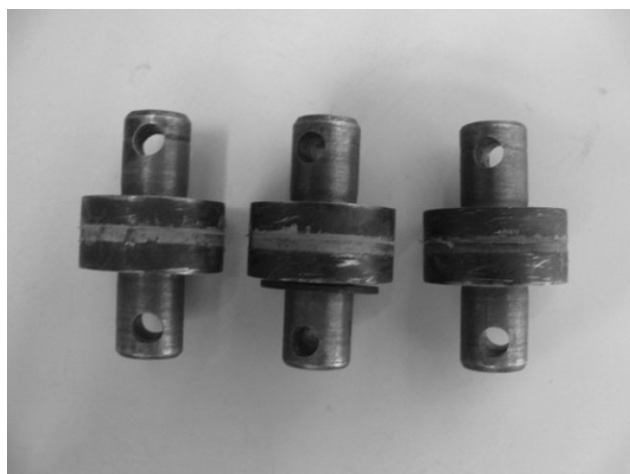
Figure 1 The bonding samples after vulcanization (without using any adhesive).
